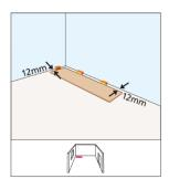
Floating floors require freedom to expand and contract without binding or rubbing on vertical surfaces. It is very important that there be enough expansion gaps between the flooring and all the walls.
