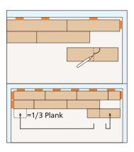
6. The width of the last row must be 1.5" or more (> 50 mm). To do this, place a full row of strips on top of the last row installed. Insert a 1/2" (12 mm) spacer against the wall, and using a full-width strip, trace a line the width of the final row from the wall. Cut strips for the final row to the designated width.
