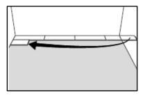
4. Fold the panel down, pressing lightly on the left. Check that the board is well joined to the top one.
