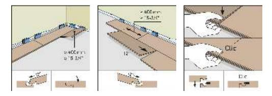
6. The **last row** of laminate flooring will almost certainly be too long, making it necessary to trim it. Remember to leave a sufficient gap along the wall. If the panels there are also too wide, they must be made narrower. Remove the blue springs at their ends and join the panels using a water-free glue.
