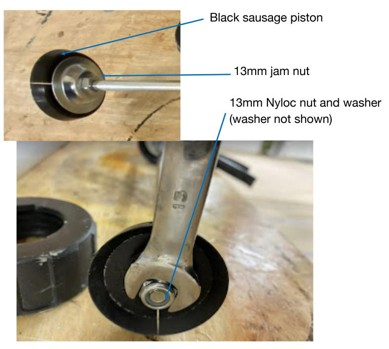
Using a 13mm wrench, remove the retaining nut, washer, and black sausage piston from the threaded push rod. (You may need a second 13mm wrench or pliers to hold the jam nut).
