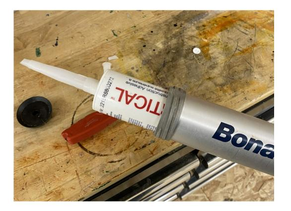
Replace the barrel, insert Bona Vertical 10 oz. tube. Thread an tighten front cap (black cuff).
