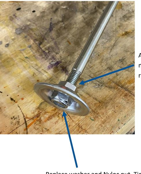
Advance the 13mm jam nut halfway up threaded rod
