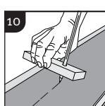
*The first and last row may need to be adjusted at an uneven wall. Copy the wall line to the first or last plank row with the shown tool, disasemble planks, adjust and reinstall.*
