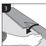
Fold the plank down in a single movement.
