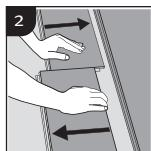
Disassemble the panels by sliding the short ends horizontally.
