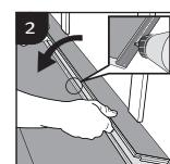
Remove the vertical locking element/hook of the plank with a chisel, put applicable glue on the locking element and push the plank horizontally together. Place wedges between last glued plank and the wall.
