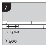
Staggered joint distance i.e. minimum distance between short ends of plank in parallel rows shall not be less than the given length.
